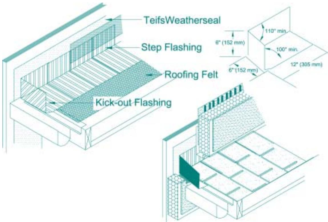
1. Kickout Flashing should extend past the edge of the roof.
