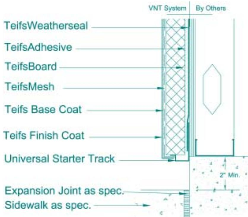
TEIFS recommends the use of high impact mesh at grade levels and all high impact areas. High impact areas utilizing 15 or 20 oz. reinforcing mesh should be noted on detail.
