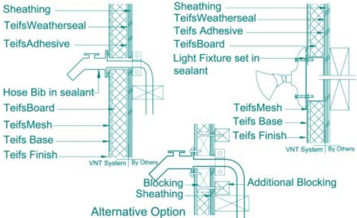
Additional blocking would be required behind the sheathing for non-wood based
