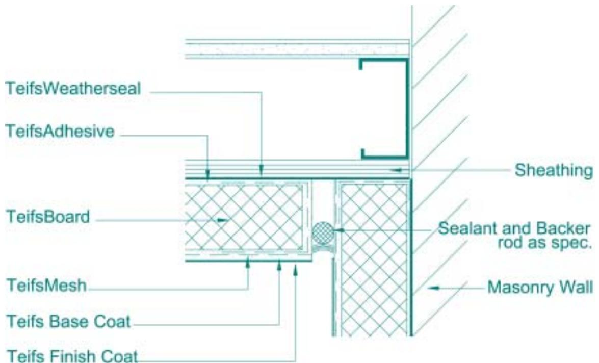
Structural engineer shall determine joint dimensions.
