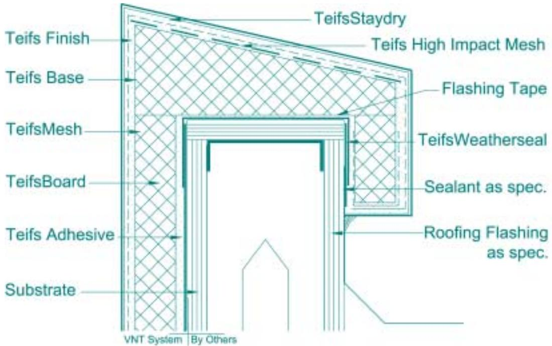
1. TEIFS requires the use of high impact mesh on parapet caps and all high impact areas. High impact areas utilizing 15 or 20 oz. reinforcing mesh should be noted on detail.
