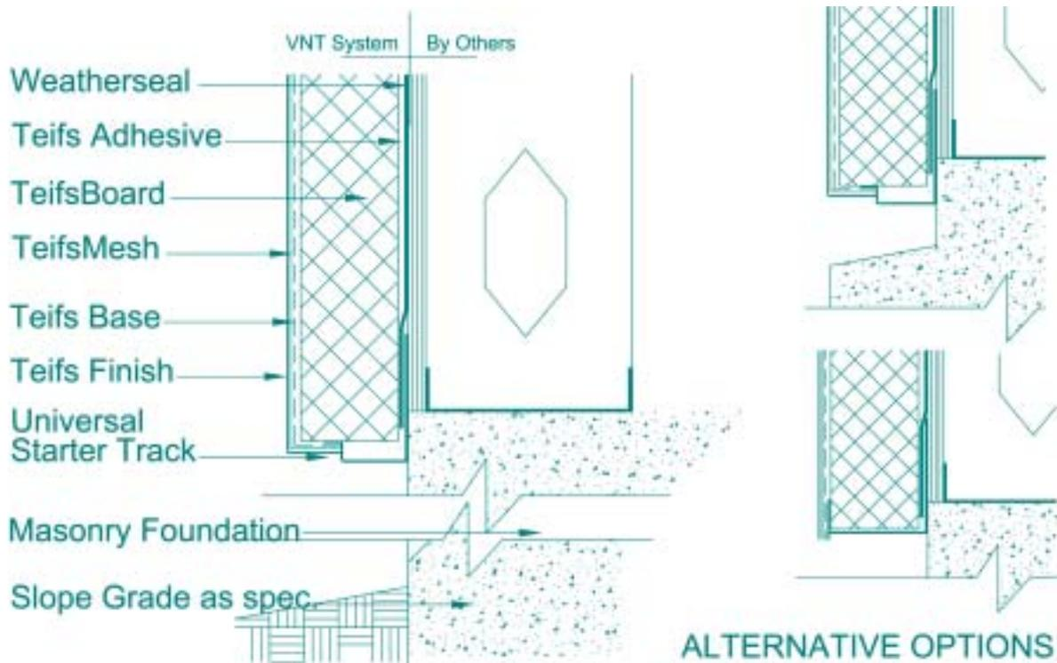
1. TEIFS recommends the use of high impact mesh at grade levels and all high impact areas. High impact areas utilizing 15 or 20 oz. reinforcing mesh should be noted on detail.
